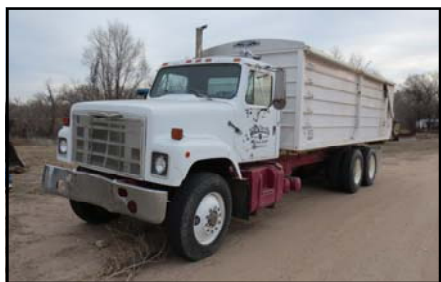
1984 IHC Truck, 22' Aulick Box, Twin Screw (Cummins 250 Engine), 11R24.5 Tires, 10-speed, 617,000 Mi.
